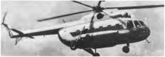
Figure 6-60. Mi-8 HIP. The standard troop helicopter in Soviet assault operations is the HIP. External racks can be mounted over the wheels to carry small arms or stretchers. Rocket pod mounts usually are mounted on either side of the cabin.
